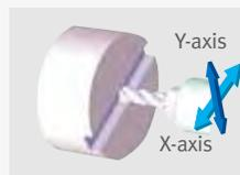
Groove finish cutting using the Y-axis
